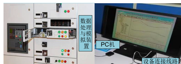
图4 负荷预测实验平台及主要设备构成 Fig. 4 Experimental platform and main equipment for load forecasting
